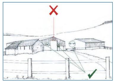
Fig. 29 Lighting should be set low down on buildings to reduce light scatter
